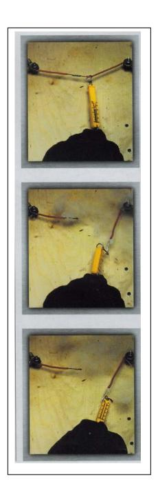
Results: The solder connections melt, wires stay intact
