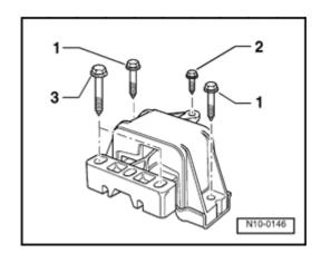
Assembly mounting, left on vehicles with manual transmission:
