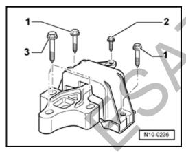
Assembly mounting, left on vehicles with automatic transmission:
