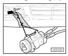
Secure the air conditioning compressor to the towing eye so that both refrigerant lines are not under tension.
